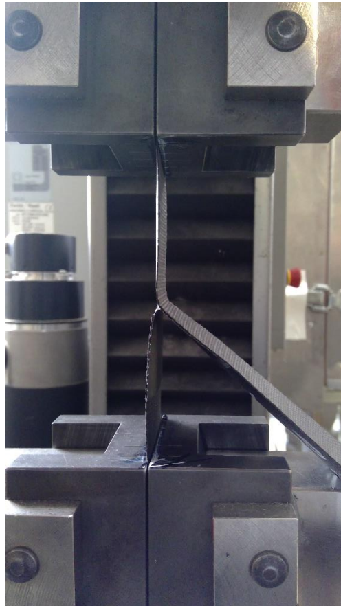
Figure 5 Peel test on joining two flexible screens with adhesive tape attachment (not visible)
