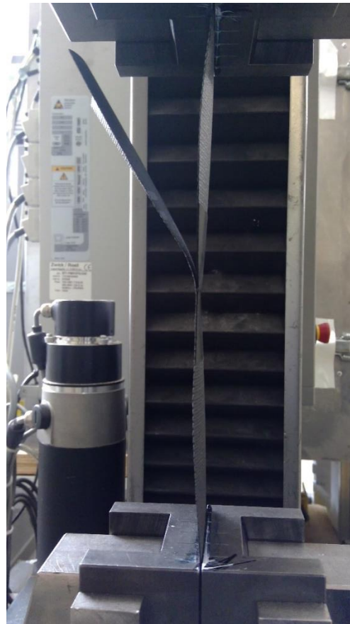
Figure 3 Shear test on junction of two flexible screens with adhesive tape attachment (not visible)
