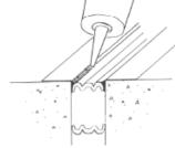
meets at butt joins, tool the excess silicone that squeezes out from the top and between the bellows. MPORTANT: Silicone left between the wrinkles
