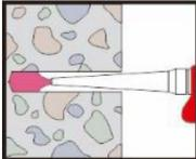
Prior to dispensing into the anchor hole, squeeze out separately the mortar until it shows a consistent grey colour, and discard non-uniformly mixed adhesive components. Start from the bottom or back of the cleaned anchor hole fill the hole up to approximately two-thirds with adhesive. Slowly withdraw the static mixing nozzle as the hole fills to avoid creating air pockets.
