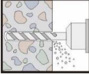
Drilling of hole with an electric drill to the diameter and depth required by the selected reinforcing bar. Drill hole diameter must be in accordance with anchor size.
