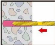
Insert the anchor with a rotary motion into the filled drill hole. Some adhesive must come out of the hole.
