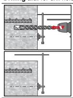
Ensure that the drill hole is parallel to the existing rebar.
