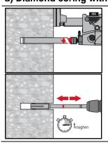
Diamond coring is permissible when suitable diamond core drilling machines and the corresponding core bits are used.
