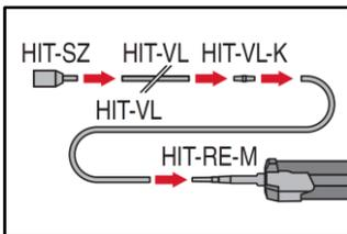
Assemble mixing nozzle HIT-RE-M, extension(s) and piston plug HIT-SZ (see Table B4, B5 or B6).
