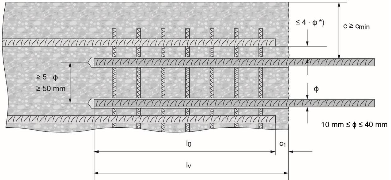
\*) If the clear distance between lapped bars exceeds  $4 \cdot \phi$ , then the lap length shall be increased by the difference between the clear bar distance and  $4 \cdot \phi$ .
