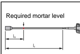
Mark the required mortar level  $l_m$  and embedment depth  $l_v$  with tape or marker on the injection extension.
