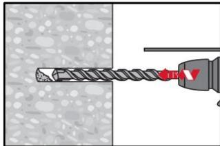
Drill hole to the required embedment depth with a hammer drill set in rotation-hammer mode or a compressed air drill using an appropriately sized carbide drill bit.
