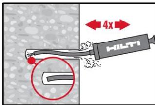
Blow again with the Hilti hand pump at least 4 times until return air stream is free of noticeable dust.
