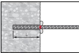
After installing the rebar, the annular gap must be completely filled with mortar.
