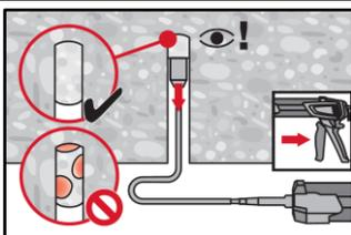
For overhead installation the injection is only possible with the aid of extensions and piston plugs. Assemble HIT-RE-M mixer, extension(s) and appropriately sized piston plug (see Table B4, B5 or B6). Insert piston plug to back of the hole and inject adhesive. During injection the piston plug will be naturally extruded out of the drill hole by the adhesive pressure.
