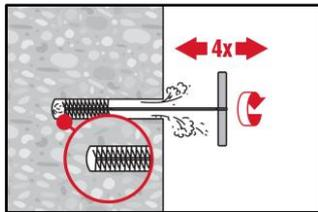
Brush 4 times with the specified brush (see Table B4) by inserting the steel brush Hilti HIT-RB to the back of the hole (if needed with extension) in a twisting motion and removing it.
