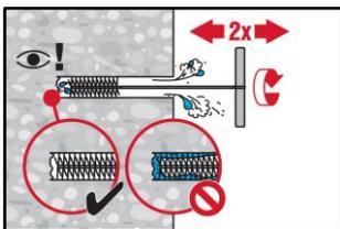
Brush 2 times with the specified brush size (brush  $\varnothing \geq$  drill hole  $\varnothing$ , see Table B6) by inserting the steel brush Hilti HIT-RB to the back of the hole (if needed with extension) in a twisting motion and removing it.
