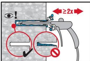
Blow again with compressed air 2 times until return air stream is free of noticeable dust and water.
