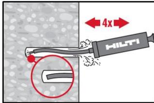
The Hilti hand pump may be used for blowing out drill holes up to diameters  $d_0 \leq 20$  mm and drill hole depths  $h_0 \leq 10 \cdot \phi$ .
