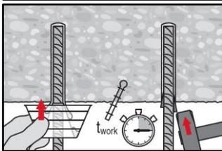
Support the rebar and secure it from falling until mortar has started to harden, e.g. using wedges HIT-OHW.
