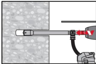
Drill hole to the required embedment depth with an appropriately sized Hilti TE-CD or TE-YD hollow drill bit with Hilti vacuum cleaner VC 20/40 (-Y) (suction volume  $\geq 57$  l/s). This drilling system removes the dust and cleans the drill hole during drilling when used in accordance with the user's manual. After drilling is completed, proceed to the "injection preparation" step in the installation instruction.
