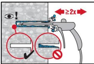
Blow 2 times from the back of the hole (if needed with nozzle extension) over the whole length with oil-free compressed air (min. 6 bar at 6 m<sup>3</sup>/h) until return air stream is free of noticeable dust and water.
