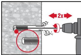
Screw the round steel brush HIT-RB in one end of the brush extension(s) HIT-RBS, so that the overall length of the brush is sufficient to reach the base of the drill hole. Attach the other end of the extension to the TE-C/TE-Y chuck.
