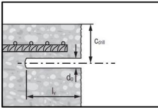
Measure and control concrete cover  $c$ .
