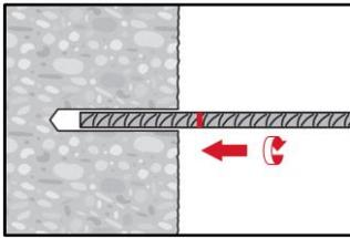
For easy installation insert the rebar into the drill hole while slowly twisting until the embedment mark is at the concrete surface level.
