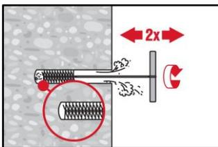
Brush 2 times with the specified brush (see Table B4) by inserting the steel brush Hilti HIT-RB to the back of the hole (if needed with extension) in a twisting motion and removing it.
