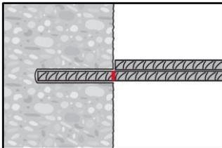
Observe the working time  $t_{work}$  (see Table B3), which varies according to temperature of base material. Minor adjustments to the rebar position may be performed during the working time.
