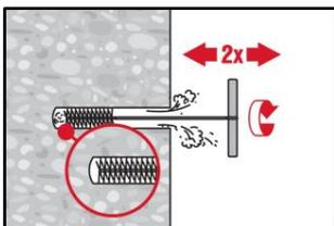
Brush 2 times with the specified brush (see Table B6) by inserting the steel brush Hilti HIT-RB to the back of the hole (if needed with extension) in a twisting motion and removing it.
