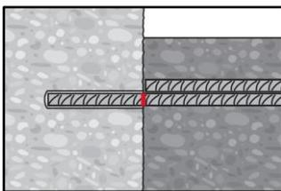
Full load may be applied only after the curing time  $t_{cure}$  has elapsed (see Table B3).
