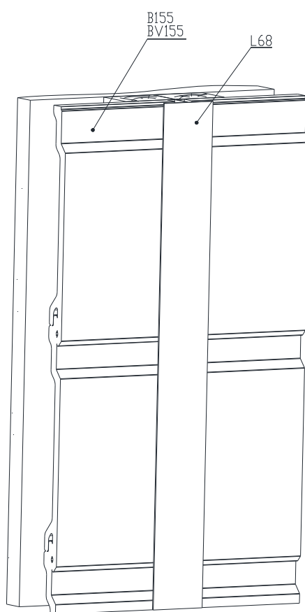
Figure 16 – Disposition horizontale – H de jonction L68
