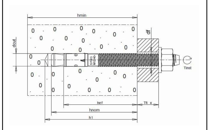
$h_{\text{ef}}\!:$  Effective anchorage depth  $h_{\text{nom}}\!:$  Installation depth
