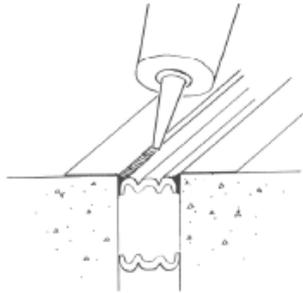
*IMPORTANT: Silicone left between the wrinkles of the bellows could constrain movement — using a caulk knife, remove excess sealant and blend what remains into the bellows.*
