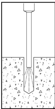
2.) Remove dust and debris from the hole using a hand pump or compressed air.
