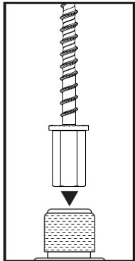
3.) Select impact wrench and mount the screw anchor head into the hex socket.
