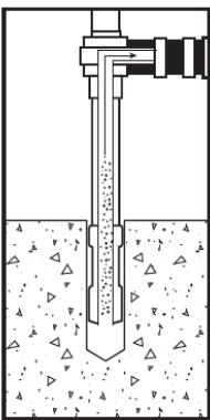
1. & 2.) Connect the hollow drill bit of proper size to a vacuum, and drill a hole into the base material to the required depth while the vac is running. The dust is removed during the drilling process.
