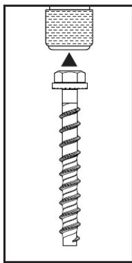
3.) Select impact wrench and mount the screw anchor head into the hex socket.
