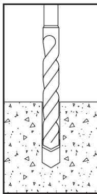
1.) Using the proper drill bit size, drill a hole into the base material to the required depth.
