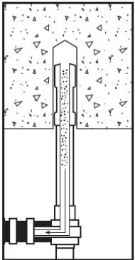
1. & 2.) Connect the hollow drill bit of proper size to a vacuum, and drill a hole into the base material to the required depth while the vac is running. The dust is removed during the drilling process.
