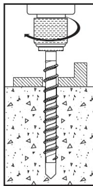
4.) Drive the anchor through the fixture into the hole at least to the minimum required embedment depth and until the head of the anchor comes into contact with the fixture.
