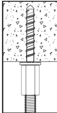
5.) Screw the threaded rod into the anchor head.
