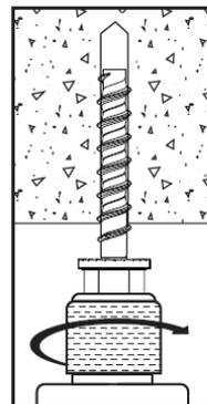
4.) Drive the anchor into the hole at least to the minimum required embedment depth and until the head of the anchor comes into contact with the base material.
