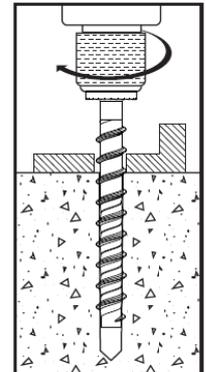
4.) Drive the anchor through the fixture into the hole at least to the minimum required embedment depth and until the head of the anchor comes into contact with the fixture.
