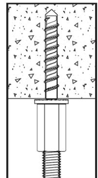
5.) Screw the threaded rod into the anchor head.
