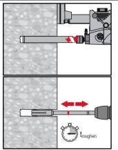
Diamond coring is permissible when suitable diamond core drilling machines and the corresponding core bits are used.
